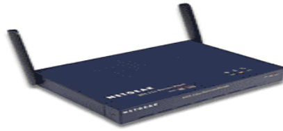
Fig 7a: Wireless Access point or Wireless Basestation
