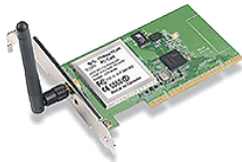
Fig 7b: Desktop PC Wireless LAN card
